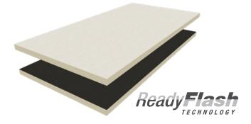
Defend-R Coated Glass is a rigid roof insulation panel composed of a closed cell polyisocyanurate foam core manufactured on-line to a premium performance coated glass facer on both sides (CGF). Manufactured using ReadyFlash<sup>®</sup> Technology, with light and dark facers. This provides the installer a choice of top side colors to better control flash-off times in fully adhered applications.
