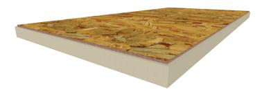
Defend-R Nail Base is a rigid roof insulation composite panel composed of a closed cell polyisocyanurate foam core manufactured on-line to a fiber reinforced facer on one side and 1/16" on the other. Defend-R Nail Base can also be manufactured off-line bonded to 5/8" OSB.
