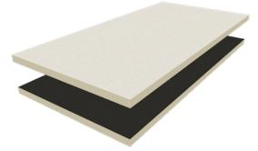
Defend-R Coated Glass is a rigid roof insulation panel composed of a closed cell polyisocyanurate foam core manufactured on-line to a premium performance coated glass facer on both sides (CGF). Manufactured using ReadyFlash<sup>®</sup> Technology, with light and dark facers. This provides the installer a choice of top side colors to better control flash-off times in fully adhered applications.
