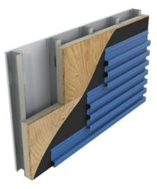
Defend-R CI Ply is an energy efficient rigid insulation panel composed of a closed cell polyisocyanurate foam core bonded to a premium performance coated glass facer on one side and 5%" or 34" fire treated plywood on the other. It is designed for use in commercial wall applications to provide both continuous insulation and an attachment substrate.
