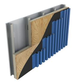
Defend-R CI Ply (Class A) is an energy efficient rigid insulation panel composed of a closed cell Class A polyisocyanurate foam core bonded to a premium performance coated glass facer on one side and 5/8" or 3/4" fire treated plywood on the other. It is designed for use in commercial wall applications to provide both continuous insulation and an attachment substrate.
