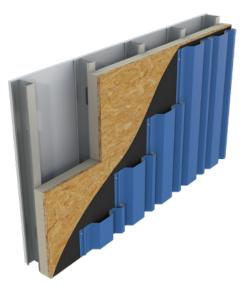
Defend-R CI Nail Base is an energy efficient rigid insulation panel composed of a closed cell polyisocyanurate foam core bonded to a premium performance coated glass facer on one side and 7/16''or 5/8'' OSB or plywood on the other. It is designed for use in Type V commercial and residential wall applications to provide both continuous insulation and an attachment substrate.
