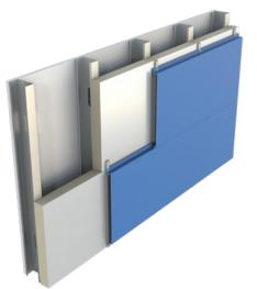
Defend-R CI Foil (Class A) is an energy efficient rigid insulation panel composed of a closed cell polyisocyanurate foam core manufactured on-line to an impermeable foil facing material. It is designed for use in commercial and residential wall applications to provide continuous insulation within the building envelope.
