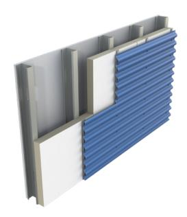
Defend-R CI Coated Glass is an energy efficient rigid insulation panel composed of a closed cell polyisocyanurate foam core combined with a premium performance coated glass facer. The panel has a light color face on one side and a dark color face on the other side. It is designed for use in commercial wall applications to provide continuous insulation within the building envelope.
