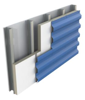
Defend-R CI Coated Glass (Class A) is an energy efficient rigid insulation panel composed of a closed cell Class A polyisocyanurate foam core manufactured on-line to premium performance coated glass facer with a light color facer on one side of the board and a dark color facer on the other side. It is designed for use in commercial wall applications to provide continuous insulation within the building envelope.
