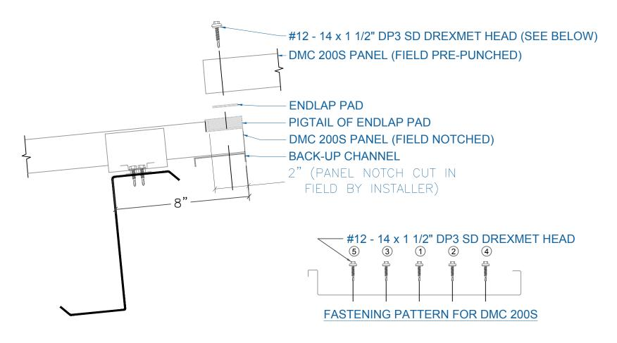
NOTE: DREXEL METALS RECOMMENDS THE USE OF PORTABLE ROLLFORMING EQUIPMENT TO AVOID END LAP CONDITIONS.
