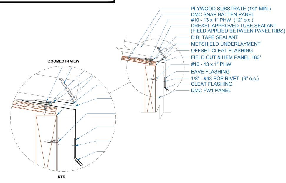
EAVE W/FLUSH PANEL Roofing Systems + Custom Fabrication
