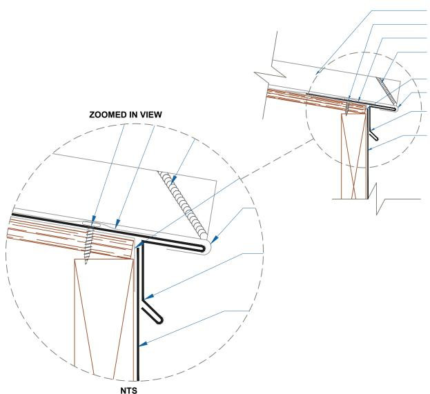
DMC SNAP BATTEN PANEL #10 - 13 x 1" PHW (12" o.c.) METSHIELD UNDERLAYMENT DREXEL APPROVED TUBE SEALANT (FIELD APPLIED BETWEEN PANEL RIBS) METSHIELD UNDERLAYMENT FIELD CUT & HEM PANEL 180°
