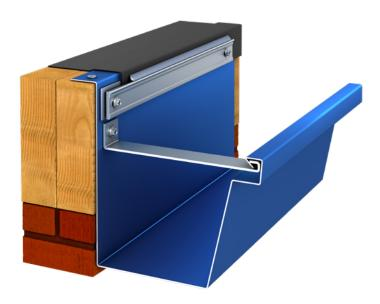
The Drexel Metals Gutter LT System is a Heavy Duty Gutter used with single-ply commercial roof systems. Our 7" Box Gutter is available in both prepainted Kynar 500°.040 formed aluminum and 24 gauge Galvalume° steel. Available in standard lengths of 10' and includes all gutter brackets (spaced 24" on center) and fasteners.
