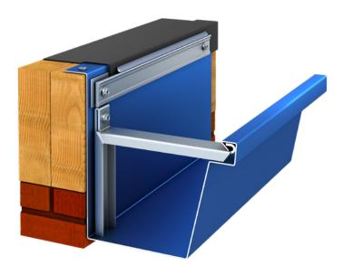
The Drexel Metals Gutter HD System is a Heavy Duty Gutter used with single-ply commercial roof systems. Our 7" Box Gutter is available in both prepainted Kynar 500° .040 formed aluminum and 24 gauge Galvalume° steel. Available in standard lengths of 10' and includes all gutter brackets (spaced 24" on center) and fasteners.
