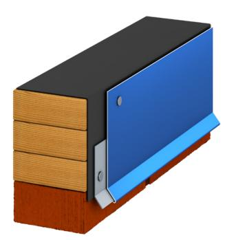
The Drexel Metals Fascia Extender is a two-part assembly that includes a continuous cleat and a decorative fascia cover for single-ply commercial roof systems. Our Extender is available in prepainted Kynar 500°.032" formed aluminum as well as 24 gauge Galvalume° steel. This product features a 24 gauge cleat with fasteners spaced at 12" on center. All products come in standard 10' standard lengths. Concealed splice plates and fasteners are included with the purchase of this product.
