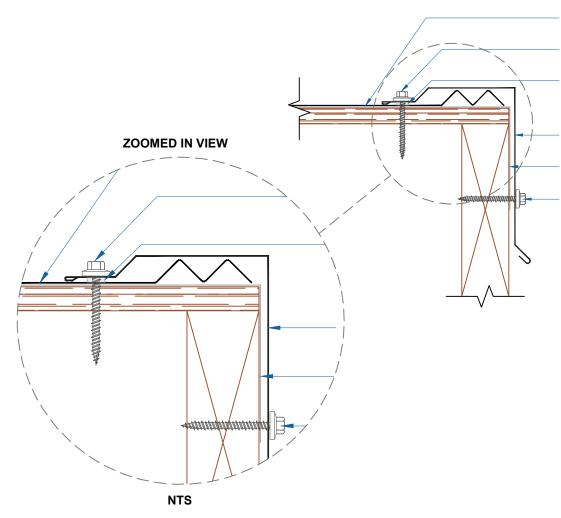
DMC 5V PANEL #10 DREXMET WOODSCREW (12" o.c.) SINGLE BEAD TAPE SEALANT
