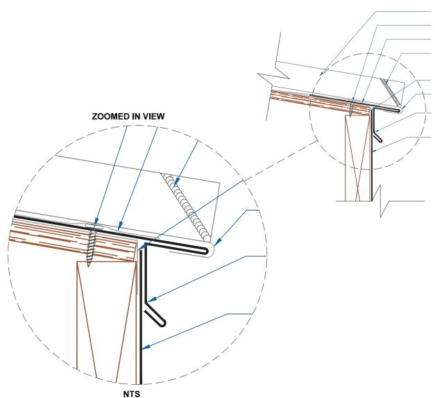
DMC 550S PANEL #10 - 13 x 1" PHW (12" o.c.) METSHIELD UNDERLAYMENT DREXEL APPROVED TUBE SEALANT (FIELD APPLIED BETWEEN PANEL RIBS) METSHIELD UNDERLAYMENT FIELD CUT & HEM PANEL 180°
