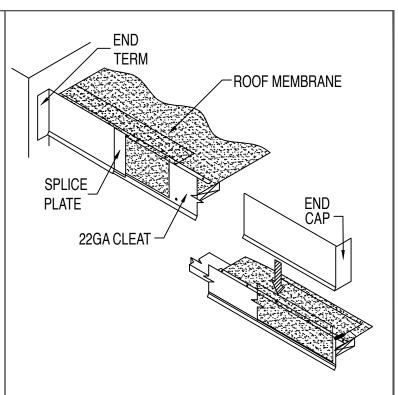
STEP 4 : Installing Gravel Stop End Caps and End Terms Install the Gravel Stop End Caps and End Terms by placing them over the Cleat, and pushing them down onto the kick out of the Cleat.
