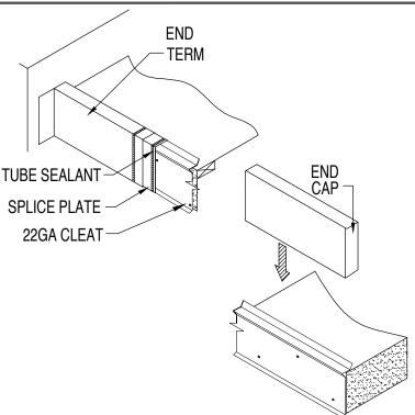
**STEP 3** : Installing Fascia Cover LT End Caps and End Terms Apply a bead of Tube Sealant inside End Cap or End Term and place a Splice Plate under each end of the End Cap or End Term. Install the Fascia Cover LT End Caps and End Terms by hooking the drip of the Fascia Cover LT End Cap or Term onto the roof side kick up of the Cleat and push down onto the lower kick out of the Cleat.
