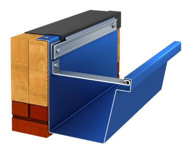
The Drexel Metals Gutter LT System is a Heavy Duty Gutter used with single-ply commercial roof systems. Our 7" Box Gutter is available in both prepainted Kynar 500°.040 formed aluminum and 24 gauge Galvalume° steel. Available in standard lengths of 10' and includes all gutter brackets (spaced 24" on center) and fasteners.
