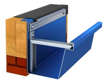
The Drexel Metals Gutter HD System is a Heavy Duty Gutter used with single-ply commercial roof systems. Our 7" Box Gutter is available in both prepainted Kynar 500° .040 formed aluminum and 24 gauge Galvalume<sup>®</sup> steel. Available in standard lengths of 10' and includes all gutter brackets (spaced 24" on center) and fasteners.
