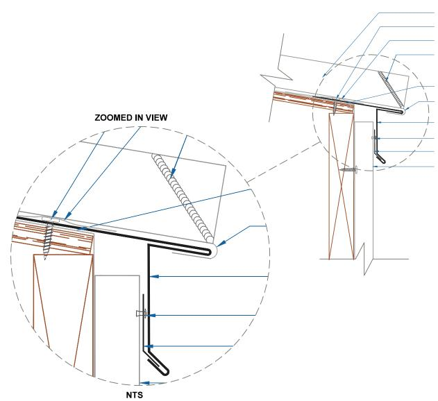
DMC 200S PANEL #10 - 13 x 1" PHW (12" o.c.) METSHIELD UNDERLAYMENT DREXEL APPROVED TUBE SEALANT (FIELD APPLIED BETWEEN PANEL RIBS)
